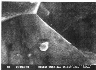
图2 Ti22 钢中晶界处含 Al 夹杂物相 Fig.2 Inclusion phase bearing Al at grain boundary in Ti22 steel
