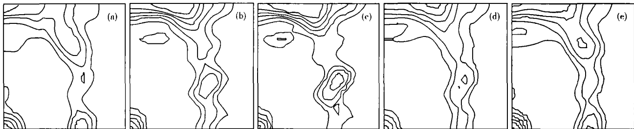
图 2 异步冷轧织构沿厚度方向的恒 \Phi = 45^\circ ODF 截面图,至快辊侧表层距离:(a) t=0 ; (b) t=0.125 mm; (c) t=0.25 mm; (d) t=0.375 mm; (e) t=0.5 mm Fig.2 ODFs constant \Phi = 45^\circ section scheme of asynchronous cold rolling texture in thickness direction; distance from fast roller side- (a) t=0 ; (b) t=0.125 mm; (c) t=0.25 mm; (d) t=0.375 mm; (e) t=0.5 mm
