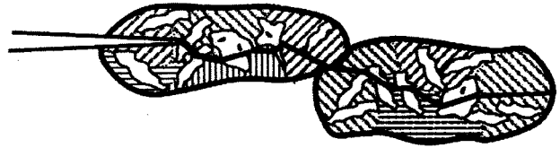
图4 Charpy冲击试样中裂纹的扩展路径 Fig.4 Crack propagation path of Charpy impact sample
