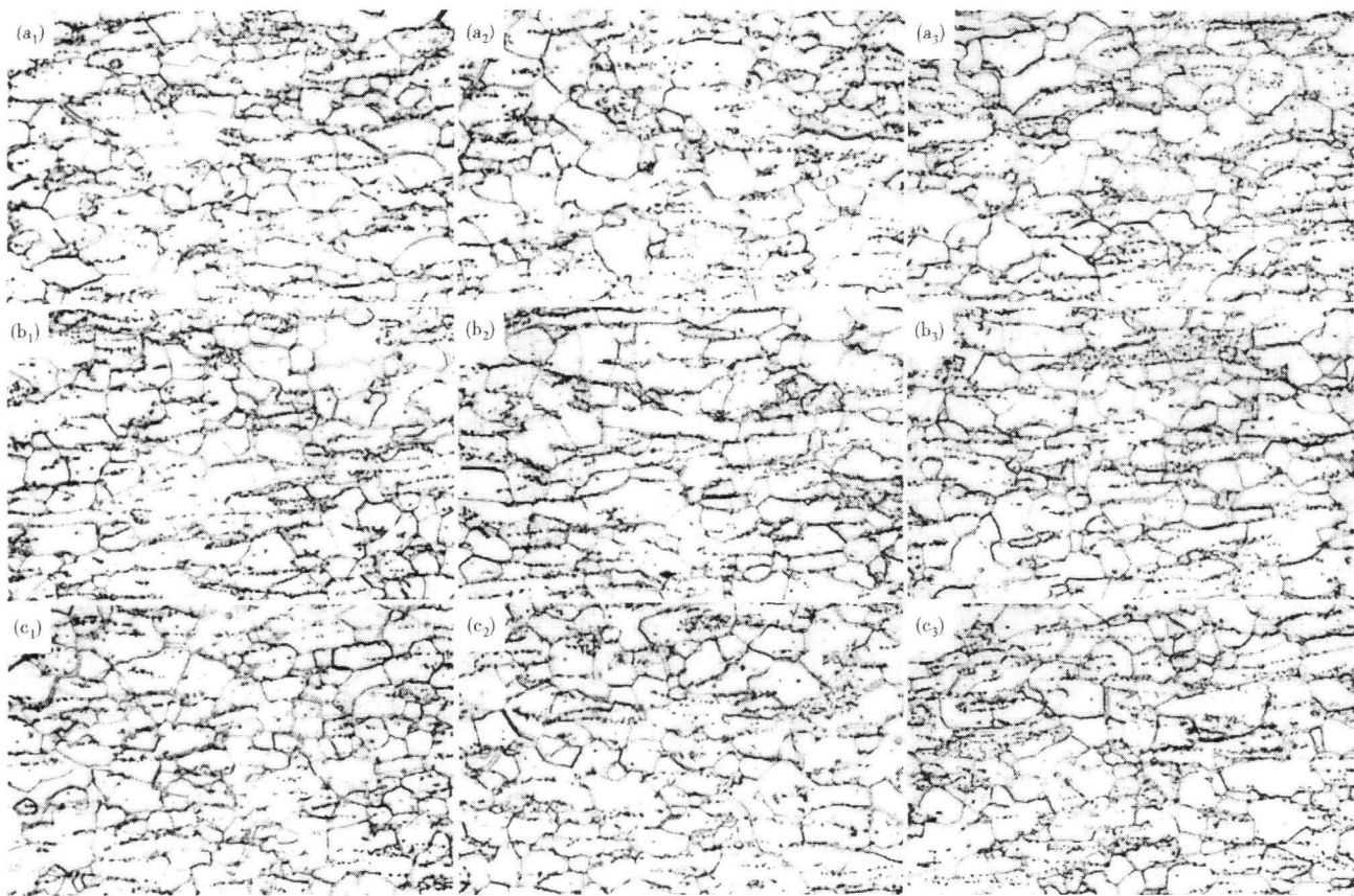
图 1 退火冷轧链条用钢板组织:650 °C 2 h(a 1 ), 4 h(a 2 ), 6 h(a 3 ); 670 °C 2 h(b 1 ), 4 h(b 2 ), 6 h(b 3 ); 690 °C 2 h(c 1 ), 4 h(c 2 ), 6 h(c 3 ) Fig. 1 Structure of cold rolled steel sheet for chain annealed at 650 °C for 2 h (a 1 ), 4 h (a 2 ), 6 h (a 3 ); at 670 °C for 2 h (b 1 ), 4 h (b 2 ), 6 h (b 3 ); and at 690 °C for 2 h (c 1 ), 4 h (c 2 ), 6 h (c 3 )
