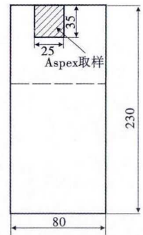
图 5 连铸坯低倍上取电解样的位置与 ASPEX 观察面 Fig. 5 Location for sampling in casting slab for electrolysis test and ASPEX observation surface on slab
