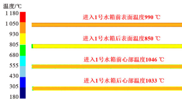
图 7 轧件进入 1 号水箱前后轧件表面和心部温度场 Fig. 7 Temperature field at the surface and core of the rolled part before and after it enters the No. 1 water tank
