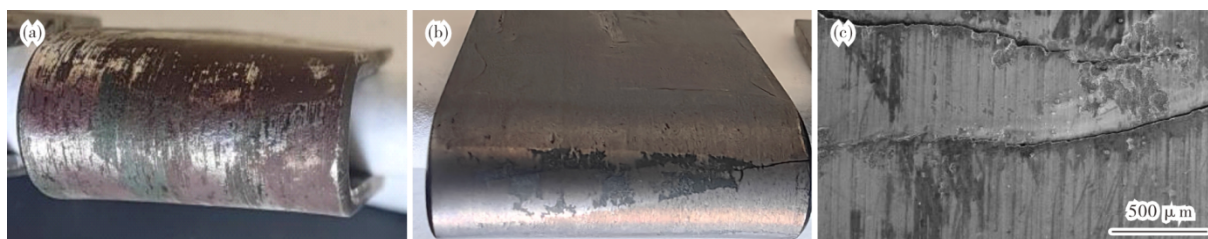
图10 应力腐蚀宏观与微观形貌: (a) 26Cr1Mo, (b) S32205, (c) S32205 微观形貌
